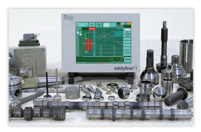
The eddyliner digital C distinguishes itself with compact design and concentration on one channel crack and grinder burn detection with one probe and combines that with the well known ibg test reliability and ease of operation. The ergonomic interface enables correct and simple operation via touch screen. All functions and test results are captured at a glance.
