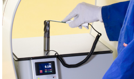
Measurement of residual magnetism of a milling cutter in the zero Gauss chamber. The demagnetized milling cutter has a residual magnetism of 0.1 \text{ A/cm} .
