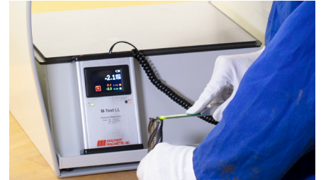
Measurement of residual magnetism of the same cutter in the earth's magnetic field. The induced fields falsify the measurement result from 0.1 \text{ A/cm} to about 2.1 \text{ A/cm}
